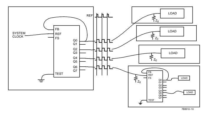
Figure 2. Board-to-Board Clock Distribution
