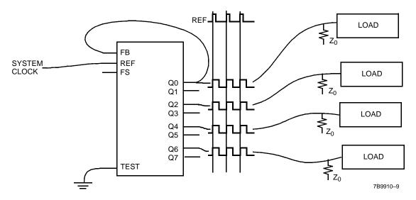
Figure 1. Zero-Skew and/or Zero-Delay Clock Driver
