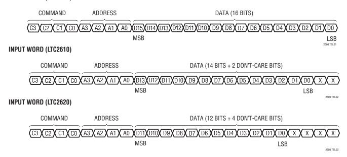
32-bit sequence. The 32-bit word is required for daisychain operation, and is also available to accommodate microprocessors which have a minimum word width of 16 bits (2 bytes).
