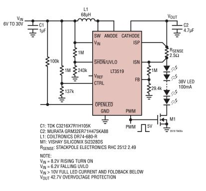
1000:1 PWM Dimming at 120Hz
