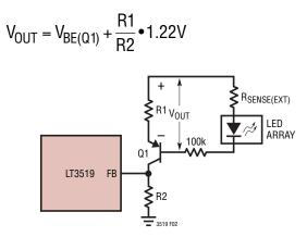
Figure 2. Open LED Protection FB Resistor Connector for Buck Mode or Buck-Boost Mode LED Driver
