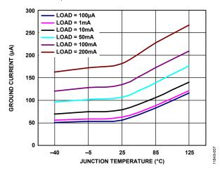
Figure 9. Ground Current vs. Junction Temperature
