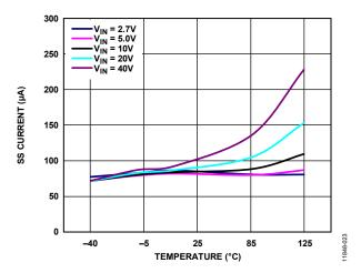
Figure 25. Soft Start (SS) Current vs. Temperature, Multiple Input Voltages ( $V_{\mathbb{N}}$ ),  $V_{\mathbb{O}UT}=5~V$
