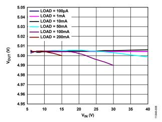
Figure 8. Output Voltage (Vouт) vs. Input Voltage (Vin)
