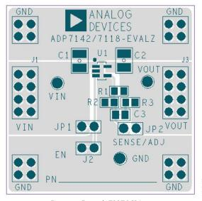
Figure 66. Example TSOT PCB Layout
