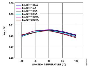
Figure 16. Output Voltage ( $V_{OUT}$ ) vs. Junction Temperature,  $V_{OUT} = 3.3 \text{ V}$
