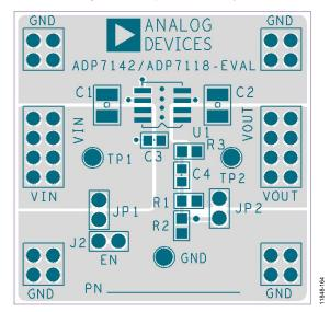
Figure 65. Example SOIC PCB Layout
