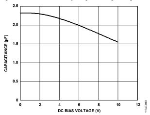
Figure 45. Capacitance vs. Voltage Characteristic
