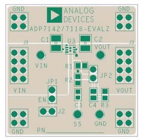
Figure 64. Example LFCSP PCB Layout
