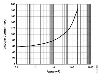
Figure 10. Ground Current vs. Load Current (ILOAD)
