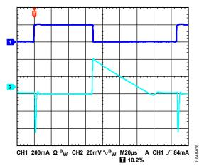
Figure 40. Load Transient Response,  $I_{LOAD} = 1 \text{ mA}$  to 200 mA,  $V_{OUT} = 1.8 \text{ V}$ ,  $V_{IN} = 3 \text{ V}$ , CH1 Load Current ( $I_{LOAD}$ ), CH2  $V_{OUT}$
