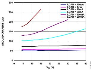
Figure 21. Ground Current vs. Input Voltage ( $V_{IN}$ ),  $V_{OUT} = 3.3 \text{ V}$
