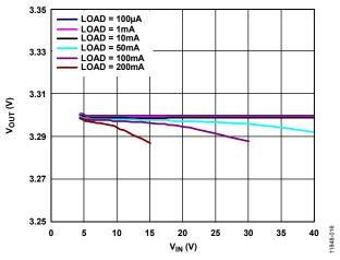
Figure 18. Output Voltage ( $V_{OUT}$ ) vs. Input Voltage ( $V_{IN}$ ),  $V_{OUT} = 3.3 \text{ V}$
