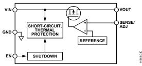
Figure 42. Internal Block Diagram
