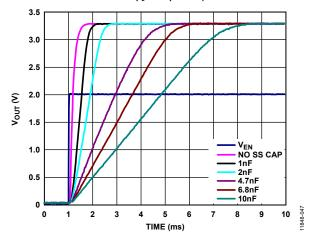
Figure 49. Typical Soft Start Behavior, Different Css
