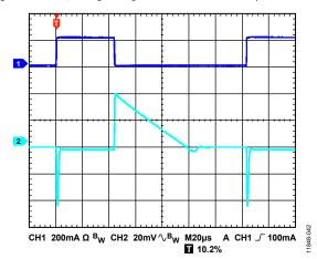
Figure 44. Output Transient Response,  $V_{OUT}$  = 5 V,  $C_{OUT}$  = 2.2  $\mu$ F, CH1 Load Current, CH2  $V_{OUT}$
