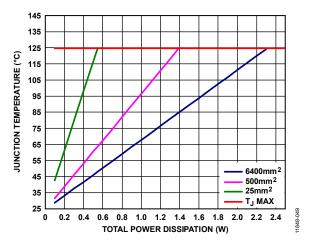
Figure 52. LFCSP,  $T_A = 25^{\circ}C$
