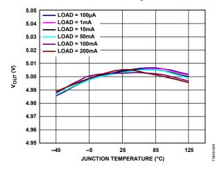
Figure 6. Output Voltage (V<sub>OUT</sub>) vs. Junction Temperature
