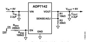
Figure 47. Typical EN Pin Voltage Divider
