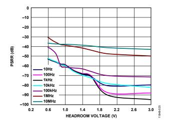
Figure 27. Power Supply Rejection Ratio (PSRR) vs. Headroom Voltage,  $V_{\rm OUT} = 1.8 \, V$ , for Different Frequencies
