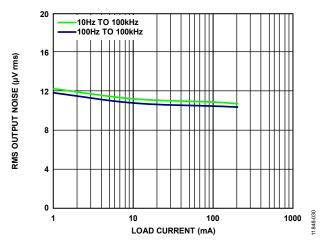
Figure 32. RMS Output Noise vs. Load Current (ILOAD)
