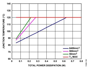
Figure 57. SOIC,  $T_A = 85^{\circ}C$
