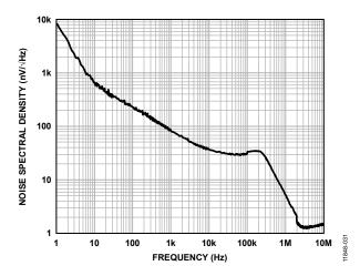
Figure 33. Output Noise Spectral Density vs. Frequency, ILOAD = 10 mA
