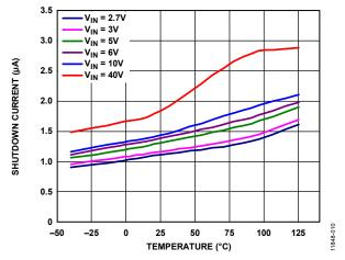
Figure 12. Shutdown Current vs. Temperature at Various Input Voltages (V<sub>IN</sub>)
