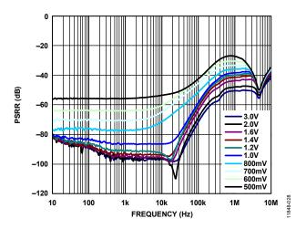
Figure 30. Power Supply Rejection Ratio (PSRR) vs. Frequency,  $V_{\rm OUT}$  = 5 V, for Various Headroom Voltages
