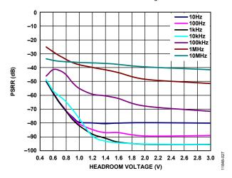
Figure 29. Power Supply Rejection Ratio (PSRR) vs. Headroom Voltage,  $V_{OUT} = 3.3 V$ , for Different Frequencies
