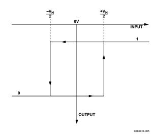
Figure 5. Comparator Hysteresis Transfer Function
