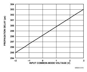
Figure 21. Propagation Delay vs. Common-Mode Voltage
