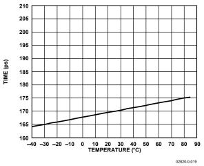
Figure 17. Fall Time vs. Temperature
