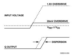
Figure 4. Propagation Delay Dispersion
