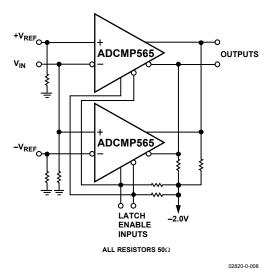
Figure 8. High Speed Window Comparator
