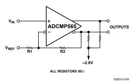
*Figure 9. Hysteresis Using Positive Feedback*
