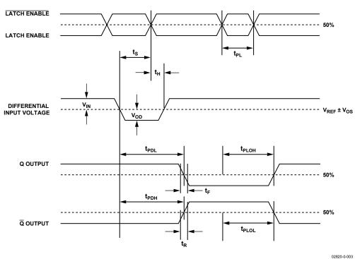
Figure 3. System Timing Diagram
