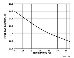
Figure 15. Input Bias Current vs. Temperature
