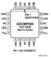
Figure 2. ADCMP565 Pin Configuration
