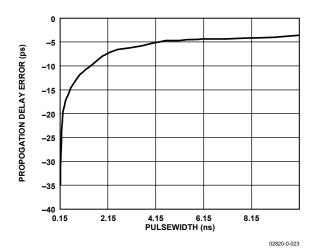
Figure 22. Propagation Delay Error vs. Pulsewidth
