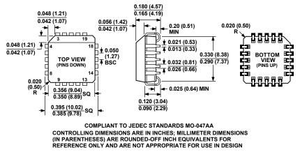
Figure 23. 20-Lead Plastic Leaded Chip Carrier [PLCC] (P-20) Dimensions shown in inches and (millimeters)
