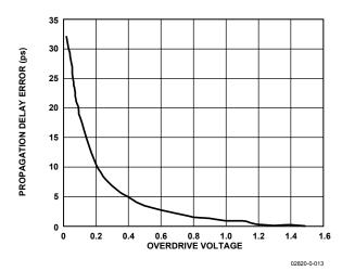
Figure 19. Propagation Delay Error vs. Overdrive Voltage
