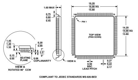
Figure 48. 100-Lead Low Profile Quad Flat package [LQFP] (ST-100-1) Dimensions shown in millimeters
