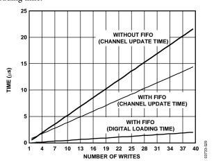
Figure 28. Channel Update Rate (FIFO vs. Non-FIFO)
