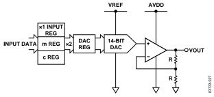
Figure 26. Single-Channel Architecture
