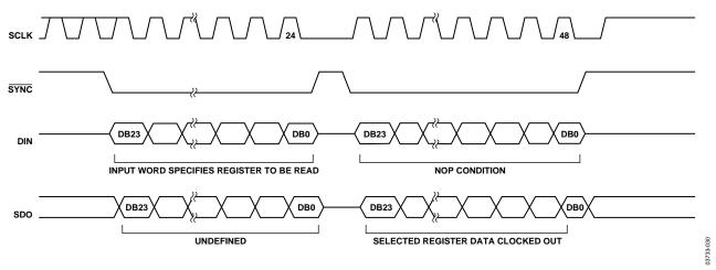
Figure 29. Serial Readback Operation
