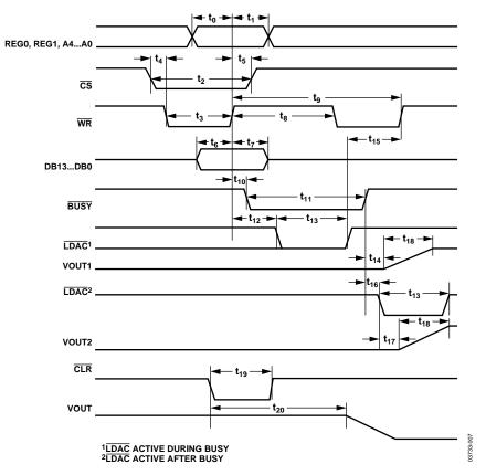
Figure 7. Parallel Interface Timing Diagram
