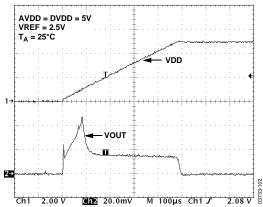
Figure 19. Exiting Hardware Power-Down
