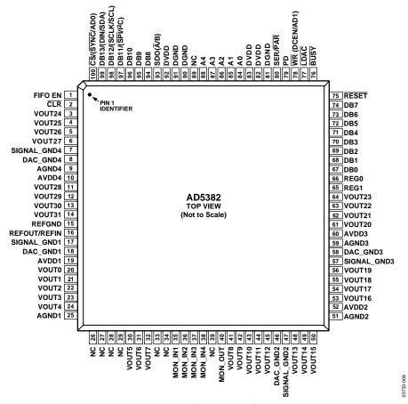
Figure 8. 100-Lead LQFP Pin Configuration
