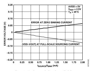
Figure 21. Headroom at Rails vs. Source/Sink Current
