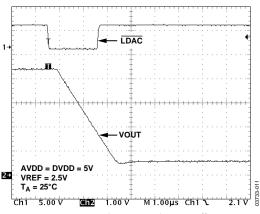
Figure 11. Slew Rate with Boost Off
