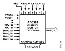
Figure 27. Channel Monitor Decoding
