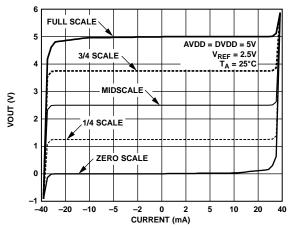
Figure 20. AD5382-5 Output Amplifier Source and Sink Capability
