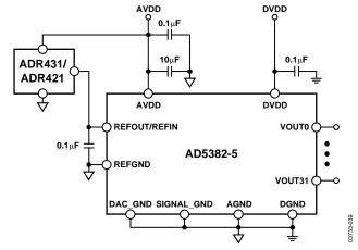
Figure 42. Typical Configuration with External Reference
