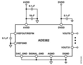
Figure 43. Typical Configuration with Internal Reference
