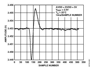
Figure 24. Adjacent Channel DAC-to-DAC Crosstalk
