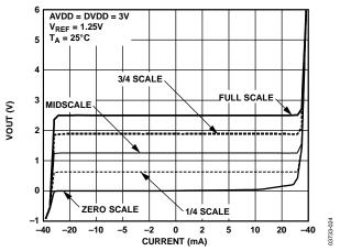
Figure 23. AD5382-3 Output Amplifier Source and Sink Capability
