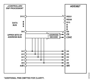
Figure 34. AD5382-to-Parallel Interface
