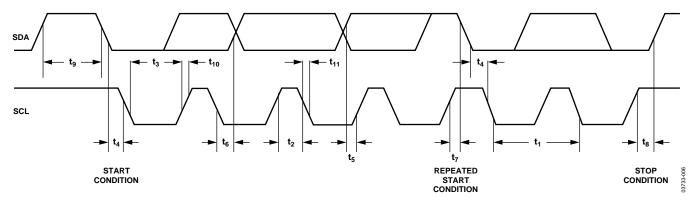
Figure 6. I<sup>2</sup>C-Compatible Serial Interface Timing Diagram
