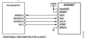
Figure 35. AD5382-to-PIC16C6x/7x Interface
