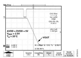
Figure 13. Slew Rate with Boost On
