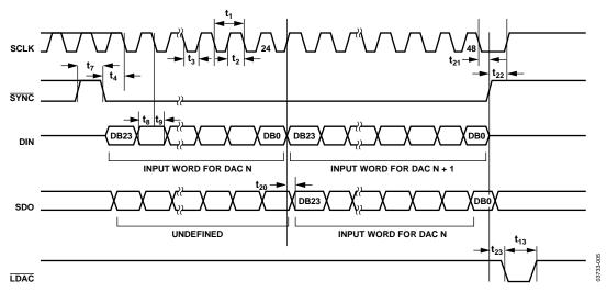
Figure 5. Serial Interface Timing Diagram (Daisy-Chain Mode)
