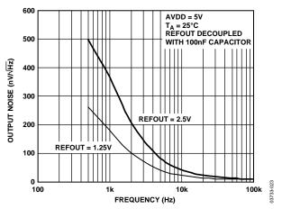
Figure 22 REFOUT Noise Spectral Density
