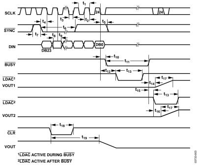
Figure 3. Serial Interface Timing Diagram (Standalone Mode)
