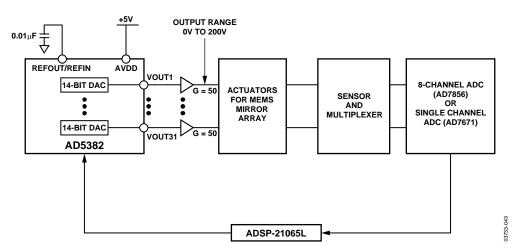
Figure 46. AD5382 in a MEMS Based Optical Switch
