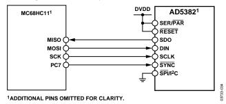
Figure 33. AD5382-to-MC68HC11 Interface
