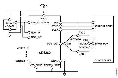
Figure 44. Typical Channel Monitoring Circuit
