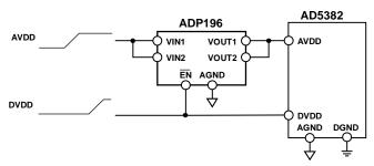
Figure 40. AVDD Power Supply Controlled by a Load Switch
