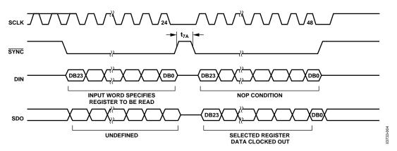
Figure 4. Serial Interface Timing Diagram (Data Readback Mode)
