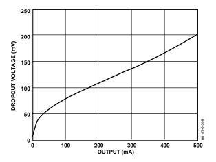
Figure 11. Dropout Voltage vs. Output Current
