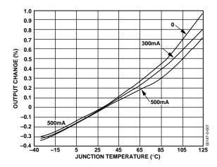
Figure 9. Output Voltage Variation vs. Junction Temperature
