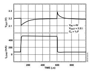
Figure 16. Load Transient Response
