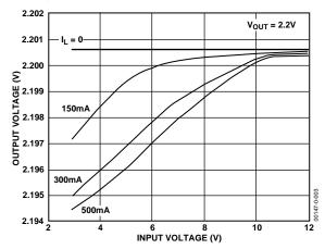
Figure 5. Line Regulation Output Voltage vs. Supply Voltage
