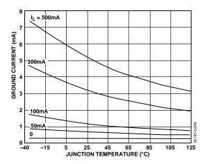
Figure 10. Ground Current vs. Junction Temperature
