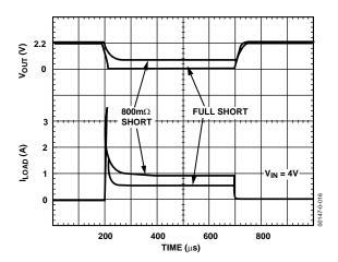
Figure 18. Short-Circuit Current
