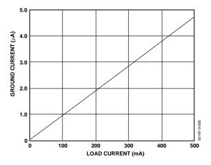
Figure 8. Ground Current vs. Load Current
