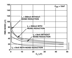
Figure 21. RMS Noise versus C<sub>L</sub> (10 Hz to 100 kHz)
