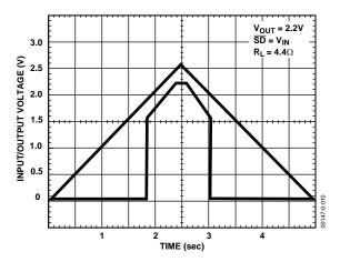
Figure 12. Power-Up/Power-Down
