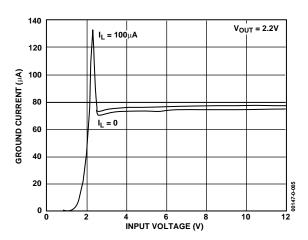
Figure 7. Ground Current vs. Supply Voltage
