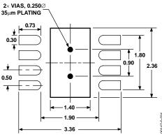
Figure 25. 3 mm × 3 mm LFCSP Pad Pattern (Dimensions shown in millimeters)
