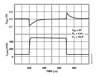
Figure 17. Load Transient Response
