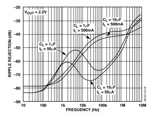
Figure 20. Power Supply Ripple Rejection
