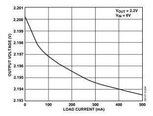
Figure 6. Output Voltage vs. Load Current
