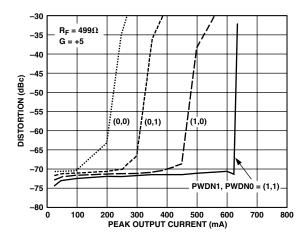
Figure 11. Distortion vs. Peak Output Current; Second Harmonic,  $V_S = \pm 12$  V,  $R_L = 10$   $\Omega$ , f = 100 kHz, Single-Ended
