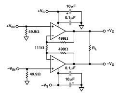
Figure 6. Differential Test Circuit; G = +10
