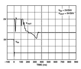
Figure 33b. Overload Recovery;  $V_S=\pm 12~V$ ,  $G=\pm 5,~R_L=100~\Omega$
