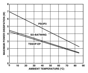
Figure 2. Maximum Power Dissipation vs. Temperature for AD8016 for  $T_J = 125^{\circ}C$
