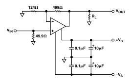
Figure 3. Single-Ended Test Circuit; G = +5
