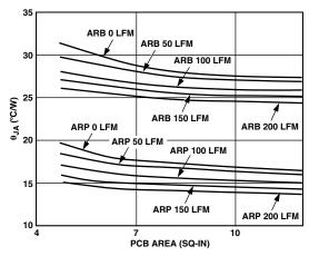
Figure 43. Junction-to-Ambient Thermal Resistance vs. PCB Area
