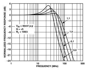
Figure 24. Frequency Response;  $V_S = \pm 6 V$ , @ PWDN1, PWDN0 Codes
