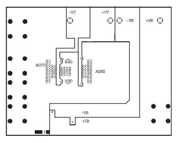
Figure 49. Power/Ground Plane
