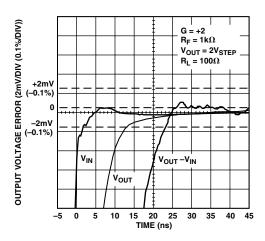
Figure 28. Settling Time 0.1%;  $V_S = \pm 12 \text{ V}$
