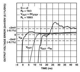
Figure 31. Settling Time 0.1%;  $V_S = \pm 6 \text{ V}$
