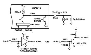
Figure 39. Shutdown and Alarm Circuit
