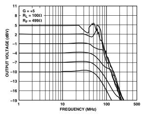
Figure 25. Output Voltage vs. Frequency;  $V_S = \pm 6 V$
