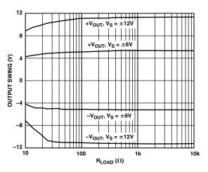
Figure 36. Output Voltage vs. R<sub>LOAD</sub>
