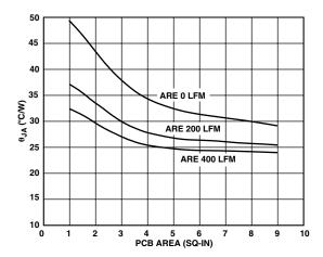
Figure 44. Junction-to-Ambient Thermal Resistance vs. PCB Area
