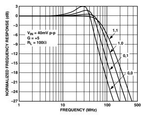
Figure 21. Frequency Response;  $V_S = \pm 12 \text{ V}$ , @ PWDN1, PWDN0 Codes
