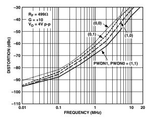
Figure 13. Distortion vs. Frequency; Third Harmonic,  $V_S = \pm 6 V$ ,  $R_L = 50 \Omega$ , Differential
