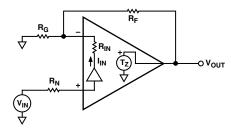
Figure 37. Simplified Block Diagram
