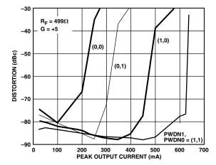
Figure 14. Distortion vs. Peak Output Current, Third Harmonic;  $V_S=\pm 12$  V,  $R_L=10$   $\Omega$ , G=+5, f=100 kHz, Single-Ended
