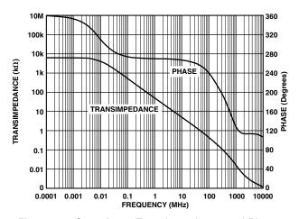
Figure 30. Open-Loop Transimpedance and Phase vs. Frequency
