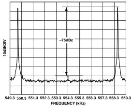
Figure 1. Multitone Power Ratio;  $V_S = \pm 12 \text{ V}$ , 20.4 dBm Output Power into 100 Ω, Downstream
