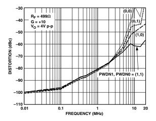
Figure 10. Distortion vs. Frequency; Second Harmonic,  $V_S = \pm 6 V$ ,  $R_L = 50 \Omega$ , Different
