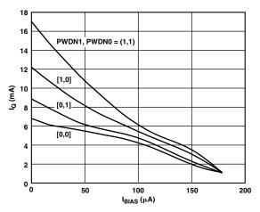
Figure 35.  $I_Q$  vs.  $I_{BIAS}$  Current;  $V_S = \pm 6 \ V$
