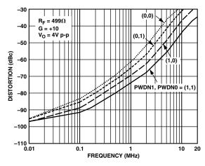
Figure 12. Distortion vs. Frequency; Third Harmonic,  $V_S = \pm 12 \ V$ ,  $R_L = 50 \ \Omega$ , Differential
