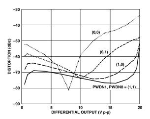
Figure 20. Distortion vs. Output Voltage, Third Harmonic,  $V_S = \pm 6 \text{ V}$ , G = +10, f = 1 MHz,  $R_L = 50 \Omega$ , Differential
