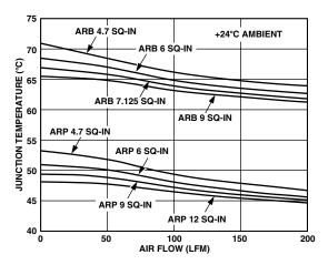
Figure 42. Junction Temperature vs. Air Flow
