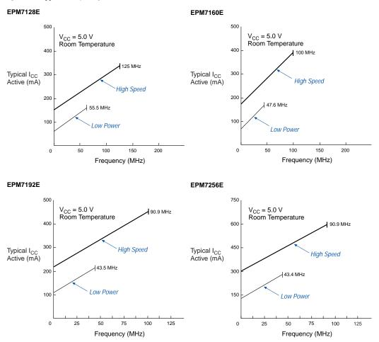
Figure 14. I<sub>CC</sub> vs. Frequency for MAX 7000 Devices (Part 2 of 2)
