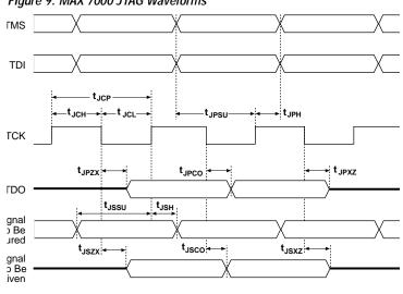
Figure 9. MAX 7000 JTAG Waveforms
