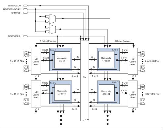
Figure 2. MAX 7000E & MAX 7000S Device Block Diagram
