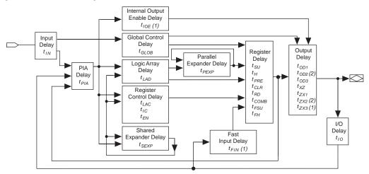
Figure 12. MAX 7000 Timing Model
