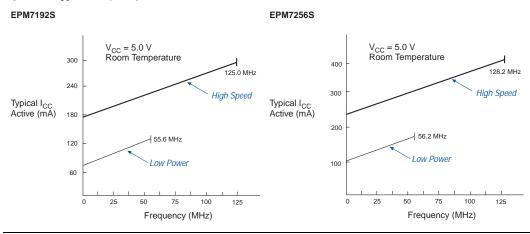
Figure 15. I<sub>CC</sub> vs. Frequency for MAX 7000S Devices (Part 2 of 2)
