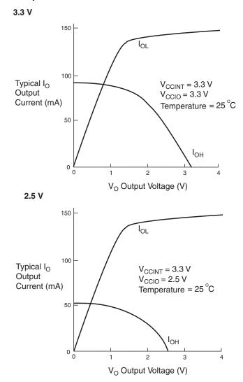
Figure 9. Output Drive Characteristics of MAX 3000A Devices
