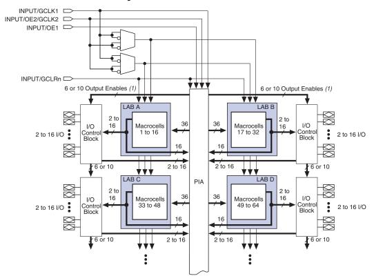
Figure 1. MAX 3000A Device Block Diagram
