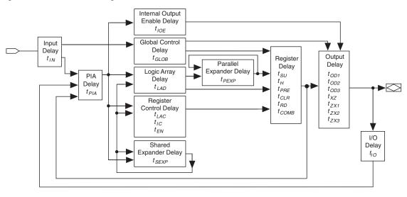
The timing characteristics of any signal path can be derived from the timing model and parameters of a particular device. External timing parameters, which represent pin–to–pin timing delays, can be calculated as the sum of internal parameters. Figure 11 shows the timing relationship between internal and external delay parameters.
