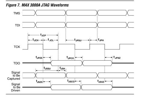
Figure 7 shows the timing information for the JTAG signals.
