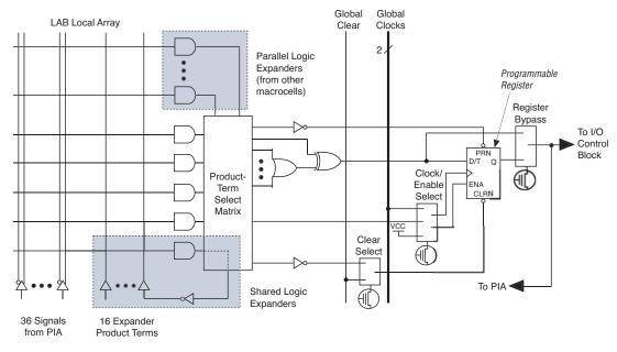
Combinatorial logic is implemented in the logic array, which provides five product terms per macrocell. The product–term select matrix allocates these product terms for use as either primary logic inputs (to the OR and XOR gates) to implement combinatorial functions, or as secondary inputs to the macrocell's register preset, clock, and clock enable control functions.
