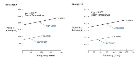
Figure 13. I<sub>CC</sub> vs. Frequency for MAX 3000A Devices
