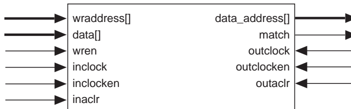
Figure 23. APEX 20KE CAM Block Diagram
