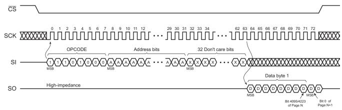
Figure 22-2. Continuous Array Read (Opcode 0BH)
