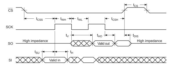
Table 19-4. Waveform 4 – RapidS Mode 3 (F<sub>MAX</sub> = 66MHz)
