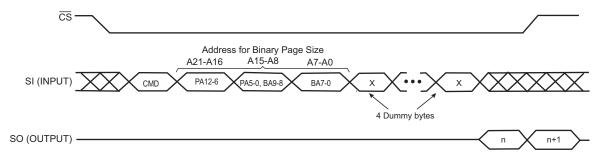
Figure 21-3. Main Memory Page to Buffer Transfer (Data from Flash Page Read into Buffer)
