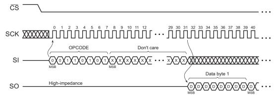
Figure 22-9. Read Security Register (Opcode 77H)
