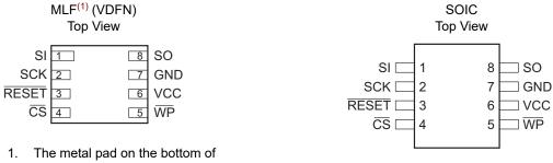
Note: 1. The metal pad on the bottom of the MLF package is floating.
