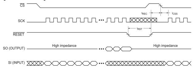
Note: The  $\overline{CS}$  signal should be in the high state before the  $\overline{RESET}$  signal is deasserted.
